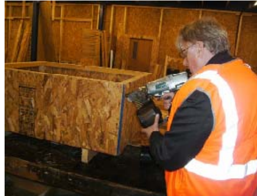
Coil Nailers for fixing Plywood to Frames Nails from 19mm-50mm Available in Ring or smooth. Plastic or Wire Collation.
