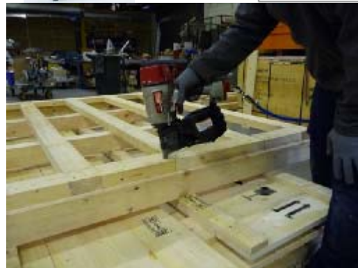
Heavy Duty Coil Nailers or Strip Nailers for fixing Frames together. Nails from 50mm-100mm. Ring, or Smooth
